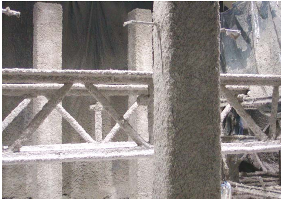
Figure 6–42. SFRM-coated steel components prior to a test.
