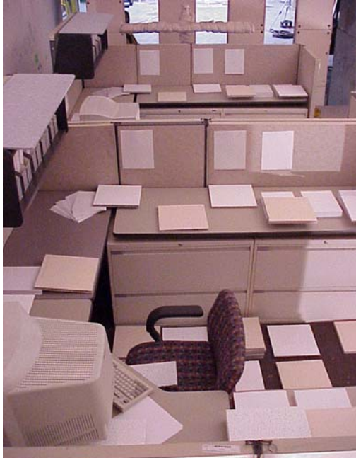
Figure 6–32. Interior view of a three-workstation fire test.
