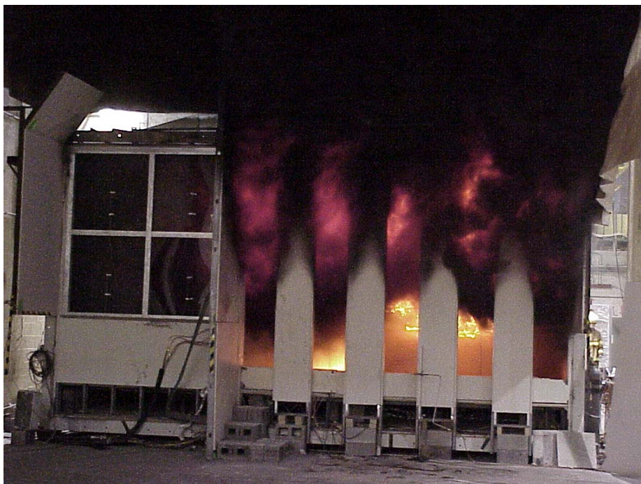
Figure 6–34. Three-workstation fire test, 2 min after the start.
